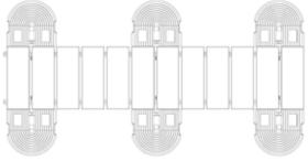
Free Standing Modules can only be used when the angle of the roof surface is less than 5 degrees inclined. These modules are held in place with the KeeGuard 100% recycled PVC counterbalances and do not penetrate the roof surface. Each counterbalance weighs 30 lbs and are  $18" \times 20" \times 3"$
